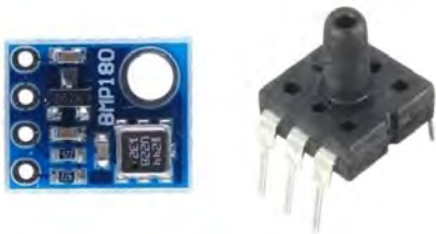
Figure 3. BMP180 Breakout GY68 next to a common air pressure sensor with a funnel-like casing.
